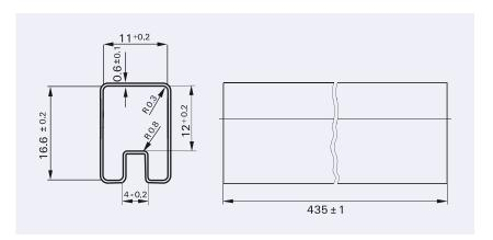
Tube dimensions 25 relays per tube 625 relays per box
